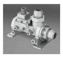
Moog model 54-164 is a cryogenic gas control valve (CVV) that provides propellant tank ullage venting for the NASA SLS Exploration Upper Stage. The pilot-operated valve vents hydrogen gas through vent thrusters during onorbit and in-transit operations to support propellant settling. The CVV also releases ullage gas overboard to help maintain stable bulk liquid propellant saturation temperature.
